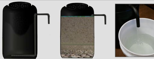
The purifier bodies are assembled from PVC pipe and HDPE plastic bodies of whatever type is locally available. Simplicity allows low cost.
